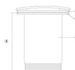
Valvula redonda con rebosadero / Round pop-up valve with overflow
